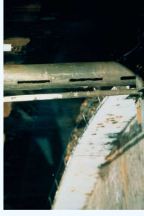
Figure 2.16: Low loss mode radar measurement can be used to virtually eliminate measurement degradation in old still-pipes.
